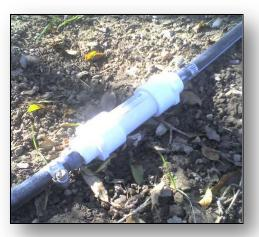
C-PROBE Soil Moisture Sensors were installed at varying soil levels to record irrigation water percolation.
