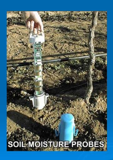
Verify the benefits of FRE-FLO™ with AquaSpy wireless soil moisture probes. Placed in the soil, they supply innovative water management solutions that measure and track in real time the movement and depth of water through the soil. Analysis software lets you control irrigations, resulting in less water use, optimum yields, improved crop quality, higher profits and enhanced water sustainability.
