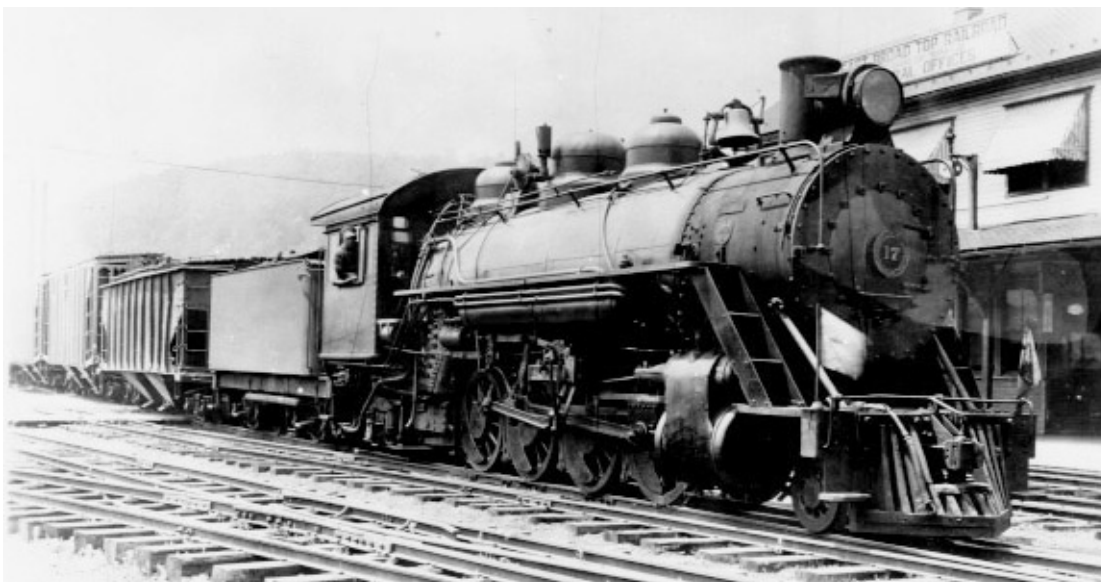
EBT 2-8-2 No. 17 passes Orbisonia station with three empty standard gauge cement hoppers riding on narrow gauge trucks during the traffic boom on the Shade Gap Branch in 1940. The empty cars will be remounted on standard gauge trucks and handed over the PRR at Mt. Union, where inbound, loaded cement hoppers will undergo the reverse process.
