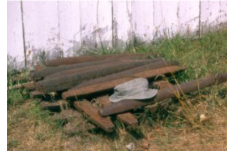
A stack of iron "pigs" outside the cast house. My hat provides some sense of scale. Each one is about 3 1/2 feet long, and weighs 90 lbs. On most charcoal iron plantations, iron pigs were reheated and pounded into wrought iron bars at a foundry.
