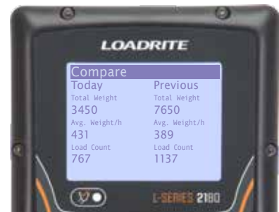
Performance data is stored to allow the operator to compare performance vs. previous, average and best shift
