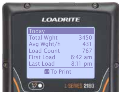
In-cab metrics feedback to the operator during the shift
