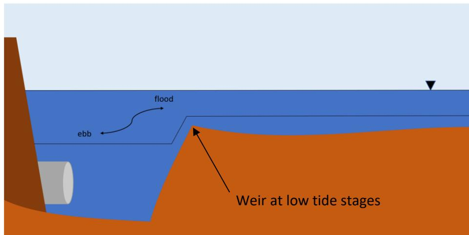
**Figure 8.** Sketch of the culvert through the embankment and into Mill Pond, the invert is at a lower elevation than the bed of the pond, which causes a weir effect over the island and into the scour pit that impedes full drainage. Note the graphic is not to scale.
