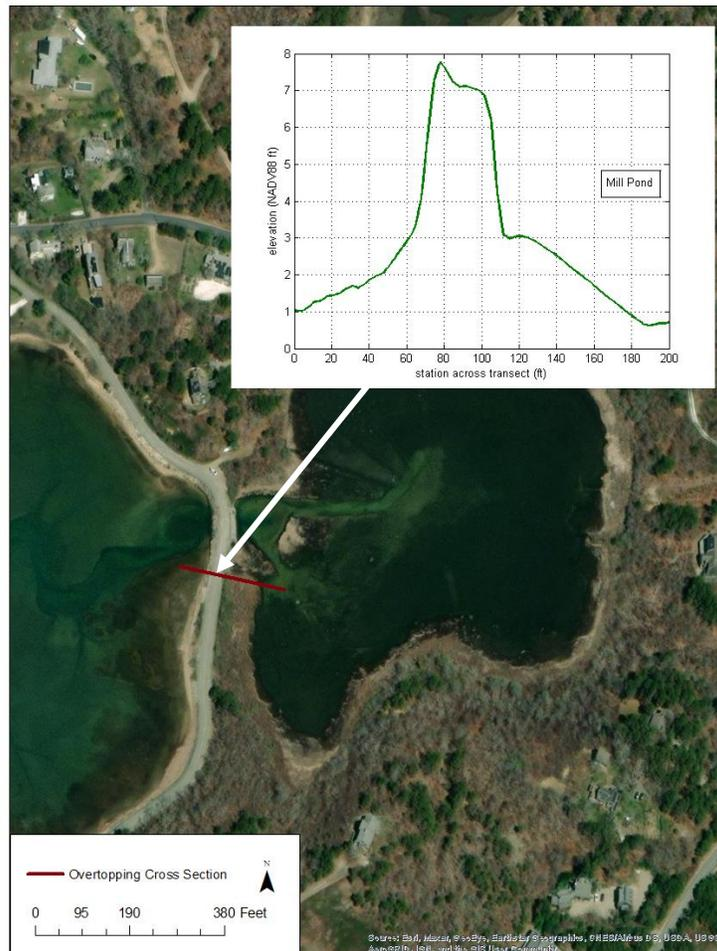
**Figure 16** Cross section of the lowest point of Mill Pond Road used to determine overtopping or wetting of the road. Note that the Mill Pond (upstream) side of the culvert is at a lower elevation than the downstream side.
