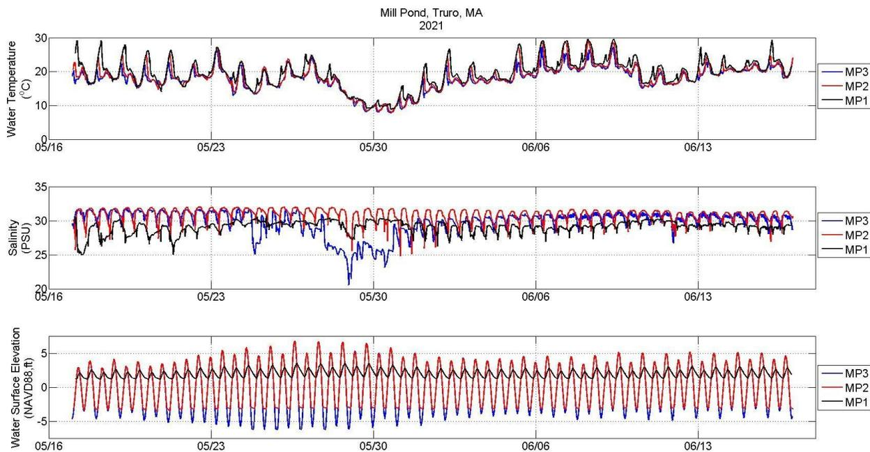
**Figure 3. Time series of the data collected by the CTD instruments. From top to bottom: Water temperature, Salinity, and water surface elevation. MP1 is in Mill Pond, MP2 in the middle basin, and MP3 in the harbor. Note that a rainstorm at the end of May decreased salinity for several days.**
