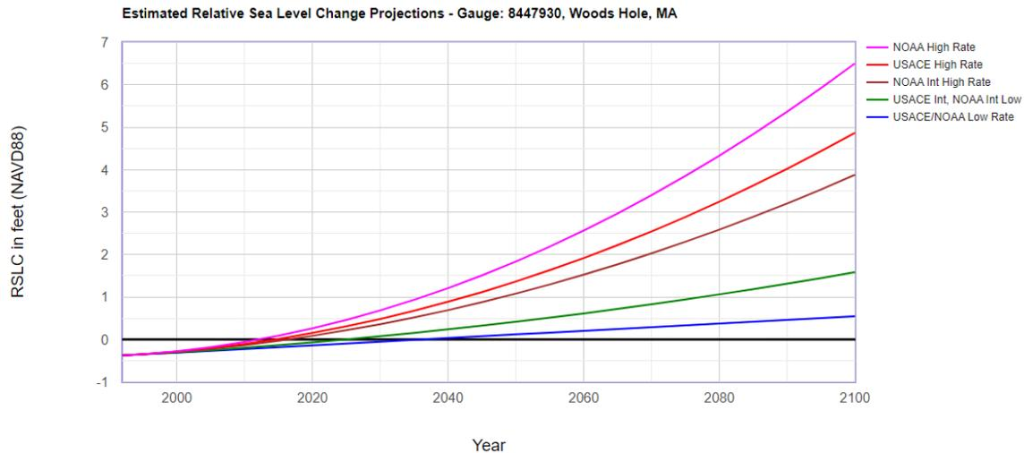
**Figure 14. USACE/NOAA sea level rise projection curves. ([Sea-Level Curve Calculator \(army.mil\)](http://Sea-Level Curve Calculator (army.mil))).**
