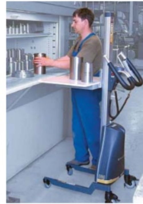
Adjust the load lifter to shelf level and remove containers by sliding them out.
