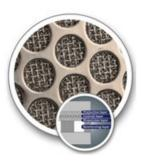
Our sintered wire mesh is available in standard configurations with up to 7 layers of media to meet the widest array of applications. The layers are compressed, sinter bonded and calendared to produce a uniform surface. Options include perforated plate or woven steel wire providing very high mechanical strength.
