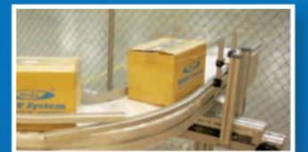
Rapid Width Adjustment (RWA) (manual/motorized)
