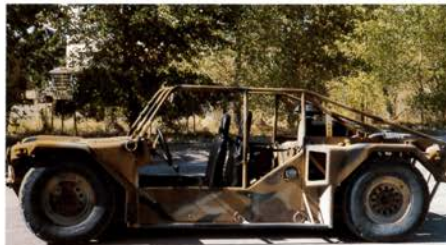
Right: The air ride system allows lowering vehicle silhouette for defoliate protection and enhancing air transport capability.
