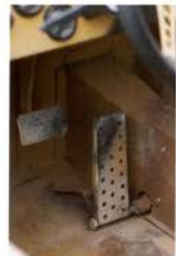
Below: Large footprint accelerator pedal permits better crosscountry control with less driver fatigue.
