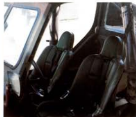
Below: Deep, bolster configured seating provides crew comfort and reduced fatigue. Fast and easy ingress/egress is possible with helmet on.
