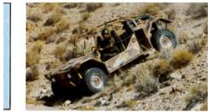
Above: Air ride system provides a progressive spring rate and is adjustable for varying loads from the driver's seat. Exceptional mobility and comfortable ride are achieved even in extremely rocky terrain.
