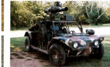
Above: Shown here with TOW installation, the LTV can also accommodate MK 19, 40 millimeter grenade launcher, 30mm and 50mm machine guns and other armament. Adequate storage space is available for other weapons and ancillary equipment.
