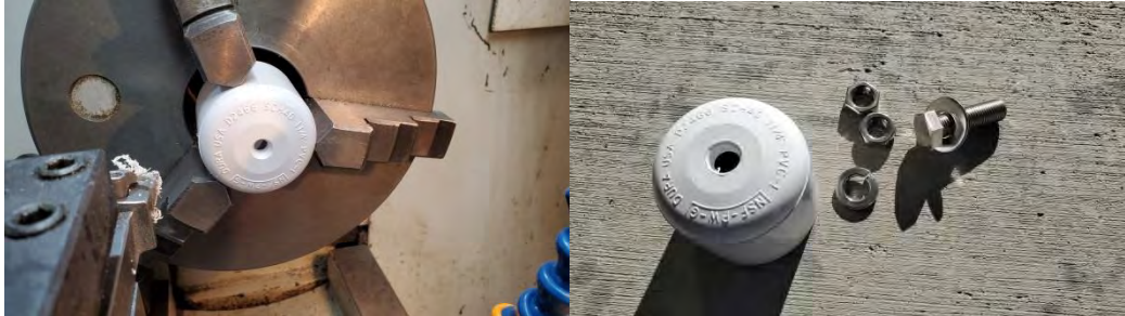
Bolt first, then flat washer, lock nut, then jam nut.
