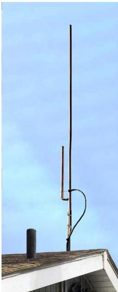
Here’s just the ticket, a tiny 12 in. high 2m staggered slot roof-topper that looks like a vent pipe. Though small, it has the gain of a J-pole. Compare size and gain in Figures 1 and 7. Which one will your neighbors notice?
