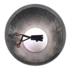
Figure 5: Internal feed point and coax balun
