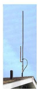
Here's just the ticket, a tiny 12 in. high 2m staggered slot roof-topper that looks like a vent pipe. Though small, it has the gain of a J-pole. Compare size and gain in Figures 1 and 7. Which one will your neighbors notice?
