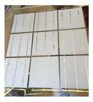
Once you have tabbed all of you cells, you need to connect them together. The front of each cell is negative and the back of the cell positive. These need to be connected like batteries in series to form a string of cells back to front. Solder the tabbing wires from the back of one cell to the front of the adjacent cell until you have completed each line. You then use the bus wire to connect the lines. The end layout should look like the attached diagram.
