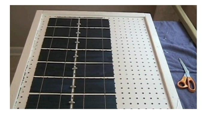
Next, after hooking all 3 strings of solar cells up in series, I was ready to get my 22 gauge wires (red and black) ready for soldering. On the ends of my leads from my gauge wires, I connected some connectors to make the process of soldering them down to the bus wire a lot easier. Watch <u>Part 7</u> of the video to see how I went about doing that.
