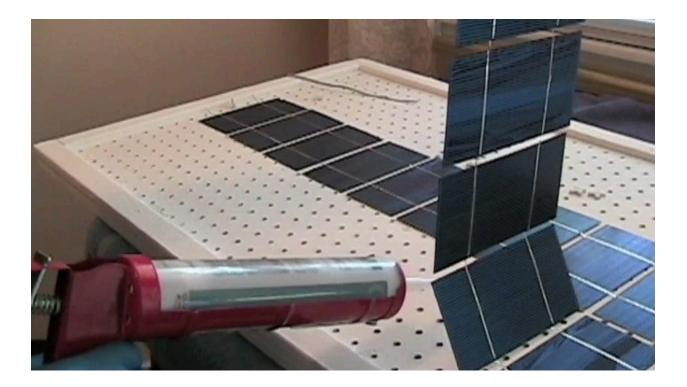
Next, it was time to glue the strings of solar cells down to the pegboard with silicon. Watch <u>Part 5</u> to see the method I used.
