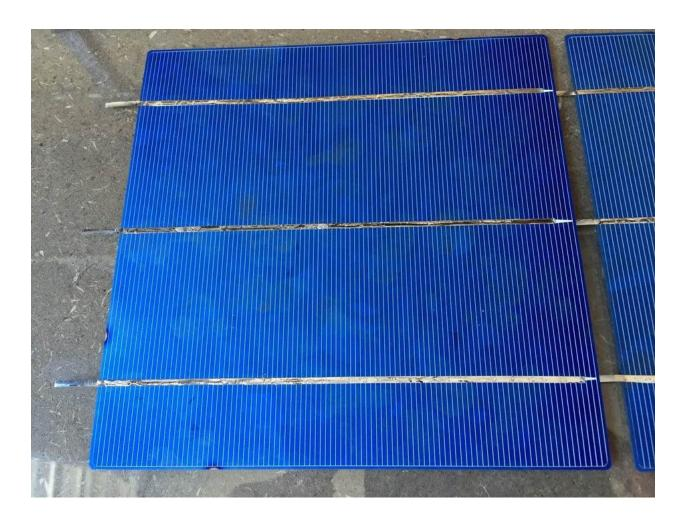
The next step, and possibly the most time consuming step, is tabbing your solar cells. You can buy pre-tabbed cells and this is recommended if you are not familiar with using a soldering iron although most solar cell suppliers will supply you with un-tabbed cells. It is not complicated once you have the correct technique but you may need to practice on one or two cells first as the tabbing wire is not easy to remove.
