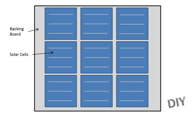
First you need to start by planning your panel layout. This is usually done according to the space you have available for the panel, you may be restricted by length or width of the panel and you can adjust the other dimensions to suite. For the 9 solar cells, a sheet of glass  $0.5m \times 6m (20'' \times 24'')$  was used and the cells were laid out as shown in the attached diagram.
