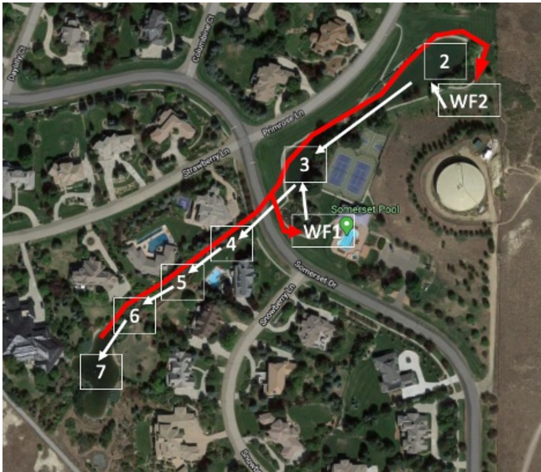
Once full, water flows from Pond 2 to Pond 7, then is pumped up to the waterfalls.
