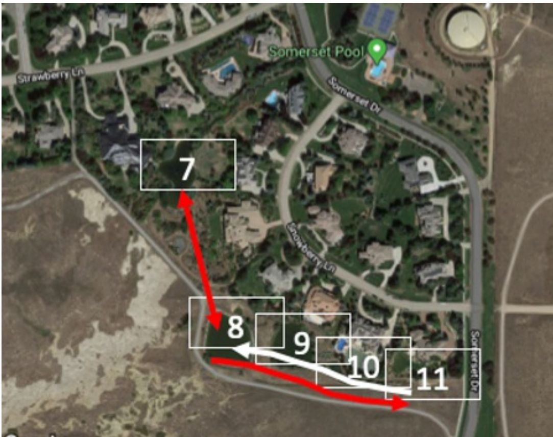
Water is pumped from Pond 7 to Pond 8, then pumped up to Pond 11
