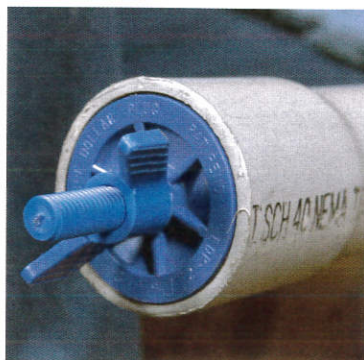
Figure 7-11. Pipe plugs are used to keep heated air within the conduit and speed up the bending process.
