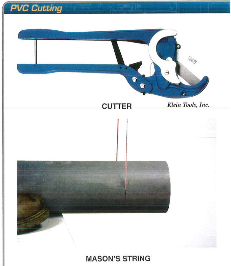
Figure 7-9. A ratchet cutter can be used to cut small-diameter PVC conduit. A mason's string makes it easy to cut larger sizes of PVC conduit in the field.
