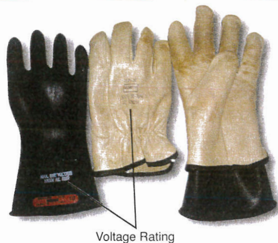
Figure 1-45 Gloves for working on live equipment must have voltage rating marks and must be tested.
