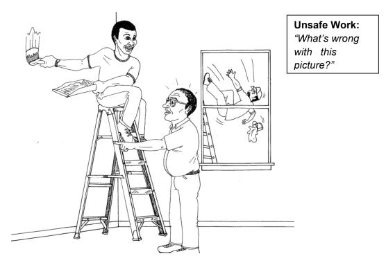
Unsafe Work: List the safety hazards inside and outside of the building.
