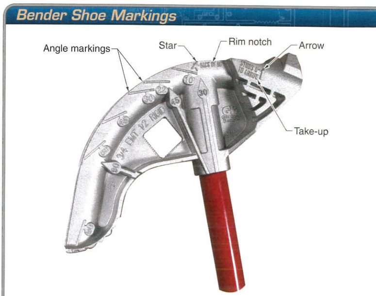
Figure 2-5. Common markings on a bender shoe include the angle markings, star, rim notch, and arrow. In addition, the take-up is often given on the bender.
