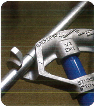
3. Align the arrow with pencil mark.
