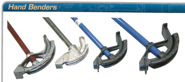
Figure 2-1. Standard hand benders are available from several manufacturers and come in a variety of sizes and configurations.
