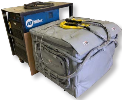
TOP LOAD OVEN WITH MILLER PROHEAT (great for heating small parts up to 1200°F)
