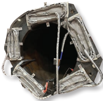
DAISY-CHAINED BLANKETS (on a large base plate for windmill)
