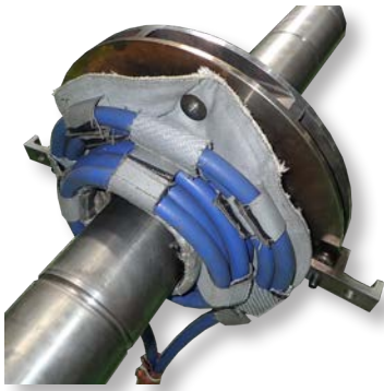
HEAT SHRINK BLANKET (rapid heat up to 600°F to remove bearing)
