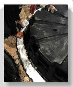
Thermal Tech & Temp's custom annealing seals work to prevent any unwanted loss of HNX gases. Our annealing seals are engineered to prevent any oxygen from coming in and causing blue steel. They also reduce airflow and the possibility of leaks in the base. We use the highest grade of insulation and superior texturized silica fabric that can withstand the wear and tear that is typically associated with the annealing process.
