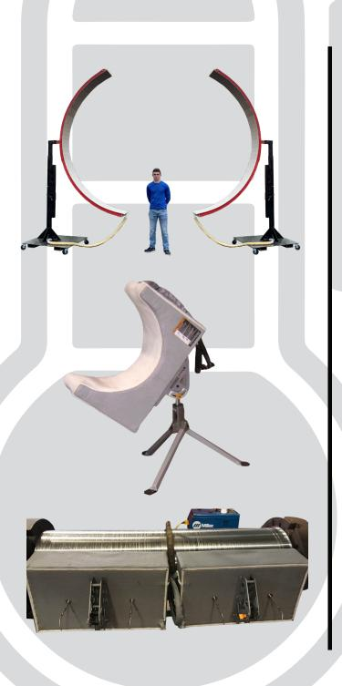
Our induction heat clams shells are custom made to fit any application. We also utilize a new style of induction coil (the electric heater) set up for the Miller ProHeat 35 Induction Heating System that focuses on pre-heating metal as it rotates. In addition, our induction heat clam shells offer a pre-heat treatment of up to 1200°F. Internal thermocouples can also be added to monitor to produce the units of temperature during the pipe's rotation.
