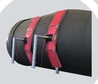
All of our induction heat clamps are custom built and can be fixed and adjusted to best suit your application. Ideally, induction heat clamps are suited for large diameter rotation when using submerged arc or manual metal arc but are also suited to small diameters
