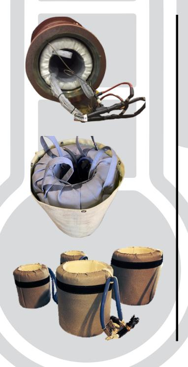
Here at Thermal Tech & Temp, our induction internal plugs are custom made to fit your application. Our plugs allow for an even pre-heat and are powered by Miller ProHeat 35. Our induction internal plugs can be inserted into bearings, vessels, and large piping for induction heating. The temperature rating of these internal plugs can be up to 1100°F.
