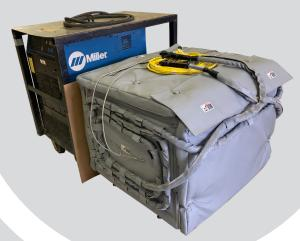
Our unique manufacturing method of induction ovens allows for a uniform preheat and stress relief of materials that you don't see in other ovens. This is especially beneficial for some metals, such as aluminum or stainless steel parts, that cannot be heat treated through direct induction. All of our induction ovens are portable units that can be moved easily and conveniently to the parts being preheated or stress relieved.
