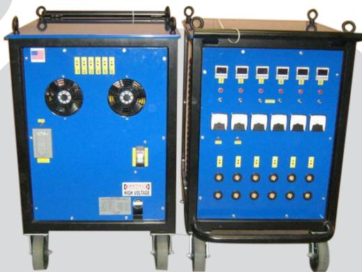
Incorporating a 1.5" tubular frame and a 1 1/4" tubed handle kick bar, the 6-way power console is fully welded, ground down, polished, and then powder coated black. The front and back panels of the machine are made of 14 gauge steel, while the side and roof panels are made from 16 gauge steel. Beneath the lid is a removable support system to prevent the lid from bending, and to also support a recorder.
