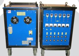
Incorporating a 1.5" tubular frame and a 1 1/4" tubed handle kick bar, the 6-way power console is fully welded, ground down, polished, and then powder coated black. The front and back panels of the machine are made of 14 gauge steel, while the side and roof panels are made from 16 gauge steel. Beneath the lid is a removable support system to prevent the lid from bending, and to also support a recorder.
