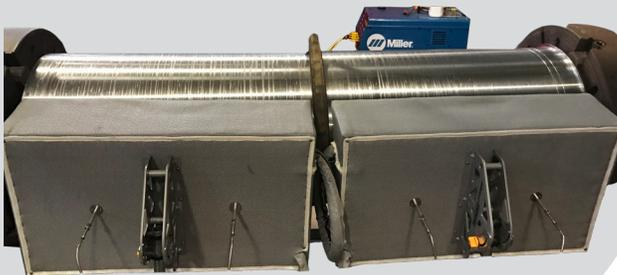
Our induction heat clams shells are custom made to fit any application. We also utilize a new style of induction coil (the electric heater) set up for the ProHeat 35 Induction Heating System that focuses on pre-heating metal as it rotates. In addition, our induction heat clam shells offer a pre-heat treatment of up to 1200°F. Internal thermocouples can also be added to monitor to produce the units of temperature during the pipe's rotation.
