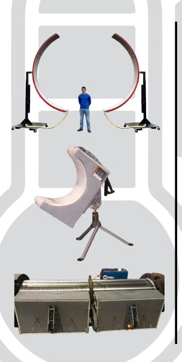
Our induction heat clams shells are custom made to fit any application. We also utilize a new style of induction coil (the electric heater) set up for the ProHeat 35 Induction Heating System that focuses on pre-heating metal as it rotates. In addition, our induction heat clam shells offer a pre-heat treatment of up to 1200°F. Internal thermocouples can also be added to monitor to produce the units of temperature during the pipe's rotation.
