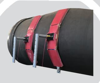
All of our induction heat clamps are custom built and can be fixed and adjusted to best suit your application. Ideally, induction heat clamps are suited for large diameter rotation when using submerged arc or manual metal arc but are also suited to small diameters
