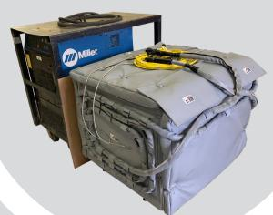
Our unique manufacturing method of induction ovens allows for a uniform preheat and stress relief of materials that you don't see in other ovens. This is especially beneficial for some metals, such as aluminum or stainless steel parts, that cannot be heat treated through direct induction. All of our induction ovens are portable units that can be moved easily and conveniently to the parts being preheated or stress relieved.
