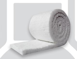
Our Soluble Fiber is a high-temperature insulation that is made from a blend of calcium, silica, and magnesium and can be exposed to temperatures up to 2200°F. Typical applications for this insulation include process furnace linings, ovens, batteries, expansion joints, boilers, and soaking pits.
