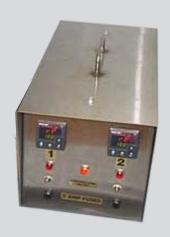
Our Twin Heat Module units will allow you to use a welder and the direct current from the welder for powering your electrical resistance heaters. In addition, our twin heat units will control the temperature and allow you to print a chart of your heat cycle for easy reference.
