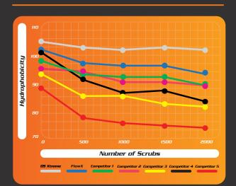
\*Car Soap (RainX) abrasion with Sponge per ASTM D2486. Contact angle measured with DI water.
