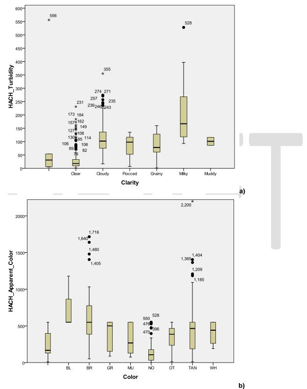
Figure 20. Comparison of Visual Observation and Field Instrument Measurements of OSTDS Sample Clarity and Color. a) Measurements of Clarity; b) Measurements of Color
