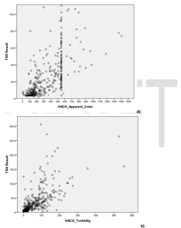
Figure 21. Concentrations of TSS Compared to Advanced OSTDS Field Instrument Measurements of a) Apparent Color and b) Turbidity. TSS-Scale is Not Fully Shown for Better Identification of Points
