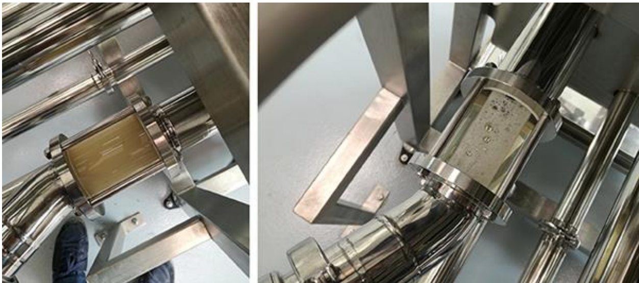
Solubilized product before and after the SMART FILTRATION stage. The product is now filtered and stabilized, ready for packaging.
