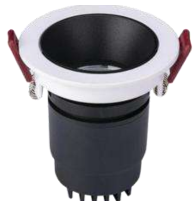
PRODUCT CODE #ALKM.024 7W/8W/12W/15W/18W COLOR:-3000K,4000K,650K CUTOUTSIZE:-55MM/75MM/95MM OUTERDIA:67MM/90MM/110MM HEIGHT :- 70MM/80MM/100MM
