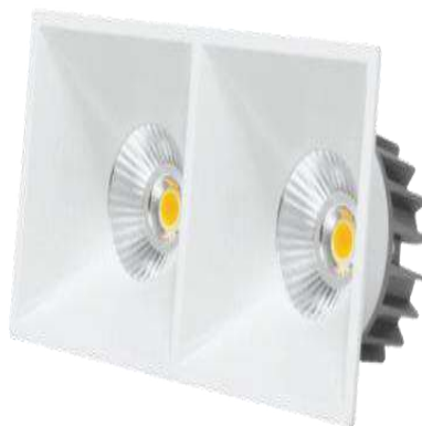
PRODUCT CODE #ALKM.023 12W*2/15W*2 COLOR:-3000K,4000K,650K CUTOUT SIZE:-155MM*77MM OUTER DIA:- 162MM*83MM HEIGHT :- 85MM
