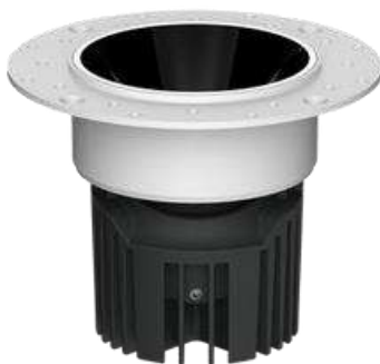
PRODUCTCODE #ALKM.025 7W/12W/15W/18W COLOR:-3000K,4000K,6500K CUTOUTSIZE:-75MM OUTERDIA:-85MM HEIGHT:-75MM/85MM/98MM
