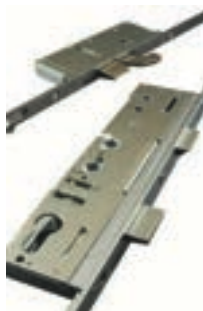
Yale The Mantis 3 Lock can be used with a Lever Lever or Lever Pad handle, the lock consists of ten locking points, four roller cams, two linear bolts, two hooks, a thumb latch and a dead bolt.
