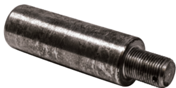
A-8013 Coultter Spindle Used To Repair Spindle On Coultter Arm. Instead Of Changing Arm, Cut Out Old Bearing Shaft, Install New Bearing Shaft And Weld In Place 3/4" Thread
