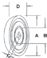
A-VLH6706 Washer, Large For 1" Axles, Cast Iron, Painted Black A: 6.437" B: 1.750" C: 1.062" D: 1.125"
