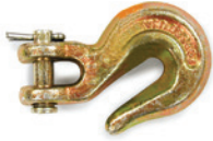
A-7B805T Hook, Grab, Clevis, Grade 70 Chain Size: .250" Hook Size: .313" Working Load Limit: 4700 lbs.
