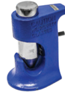
A-4266001 Crimping Tool, Hammer-Style Can be used w/ hammer or vise. Crimps terminals 8 ga. to 6/0 ga.
