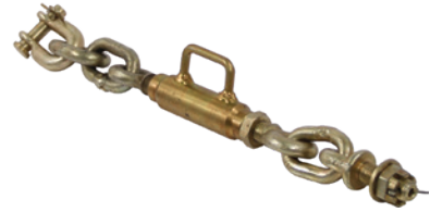
A-159350 Check Chain Stabilizer Fits most compact tractors 15 HP to 40 HP. Adjustable: 11.750" - 13.500" Body Length: 3.500" Pin Diameter: 7/16" Thread: M14-1.5
