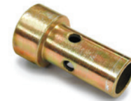
A-HB101 Bushing, Hitch, Cat II & III Inside Diameter: 1.125" Outside Diameter: 1.437"
