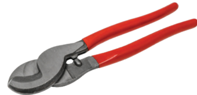
A-4275001 Cable Cutter Heavy duty 9" long, made of forged steel, has insulated grips. Cuts 8 ga. to 3/0 ga.
