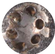
Injector after one P.i. treatment.
