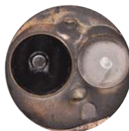
Cylinder head after one P.i. treatment.
