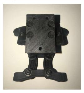
Next attach the bulkhead to the new carbon fiber chassis with the three screws and nuts provided by ERC.
