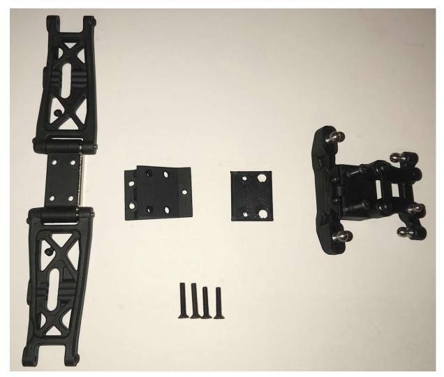
Using 2 – 3x18mm and 2 – 3x16mm flat head screws, attach the ERC Bulkhead and plate to the AE bulkhead and ball stud mount making sure the 30-degree bulkhead option is chosen for the standard setup. Make sure you get these tight without stripping. Then attach front gull wing arms, hinge pins and hinge pin brace before attaching to ERC CF Chassis.
