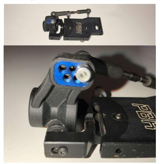
Use the zero arm mount inserts in both the C and D plates. Use 2 ERC provided spacers in front of the Plan B arms on the rear hinge pins to assemble the rear arms, rear hubs, and axles to the chassis.
