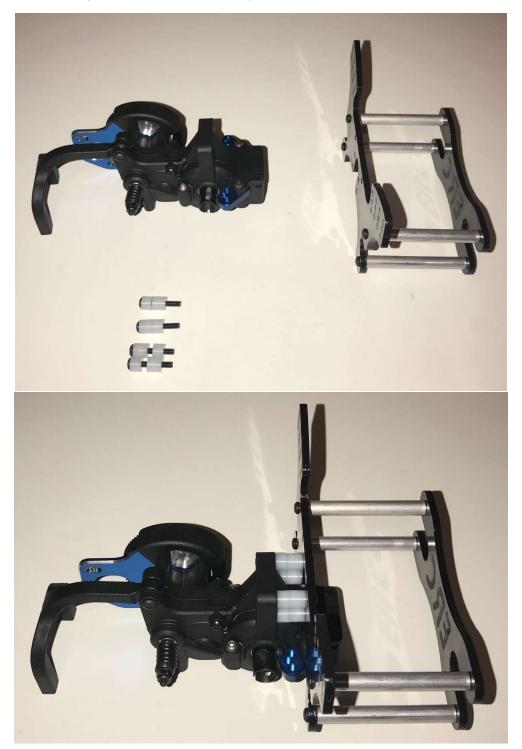
Install transmission with waterfall to ERC Carbon Fiber chassis.
