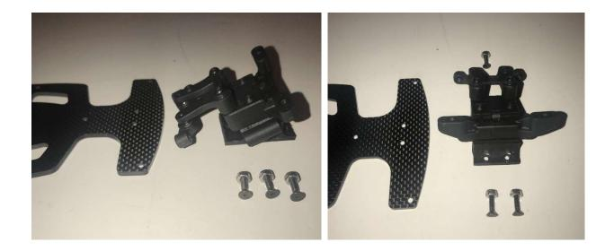
**NOTE:** Picture does not show arms attached but before you attach bulkhead assembly to chassis you may need to grind off some of the underneath side of the ball stud mount to make the arms move freely and install the arms before attaching to chassis.
