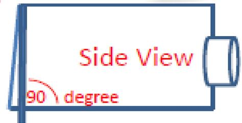
Lip is 90 deg to bottom and front spillway is about 1/2 thru lip which eliminates water drip back
