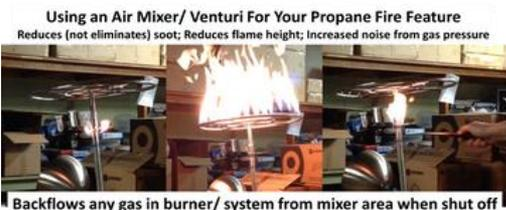
Backflows any gas in burner/ system from mixer area when shut off
