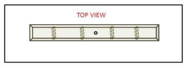
Last Step: Fill in Sides of Trough with 2" Hardie Board Strips to Cover Wood 2x4 Sides. Drill 1" Hole for Mounting Linear (Long) Burner. Attach a few more 2x4's every 1 - 1.5 ft across the bottom of the trough (for added support for rocks/ glass)..
