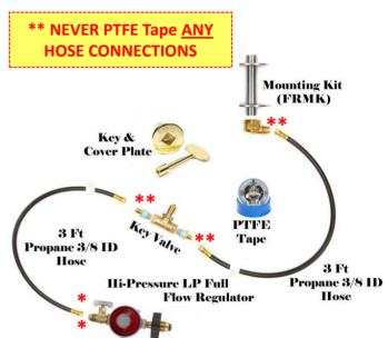
If Key Valve on ANY Deluxe kit is Going Thru 3" or Thicker Brick/ Paver; Need to Order Key Extension & Coupling (KEY12B/C & PHA12FF) \$14 / \$6
