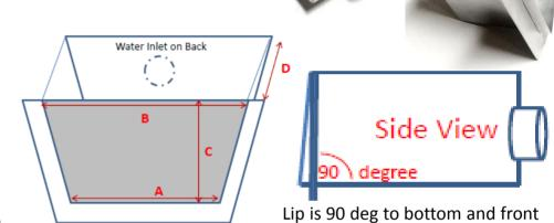
Lip is 90 deg to bottom and front spillway is about ½ thru lip which eliminates water drip back
