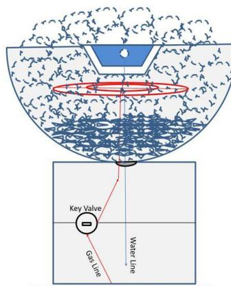
Pea Gravel in bottom of bowl to allow drainage up to the burner and avoid gas ponding. From just below the burner to the top is larger lava rocks or glass.
