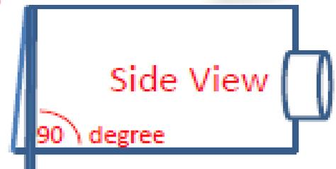
Lip is 90 deg to bottom and front spillway is about 1/2 thru lip which eliminates water drip back
