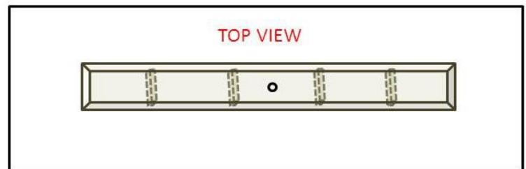
**Last Step:** Fill in Sides of Trough with 2" Hardie Board Strips to Cover Wood 2x4 Sides. Drill 1" Hole for Mounting Linear (Long) Burner. Attach a few more 2x4's every 1 – 1.5 ft across the bottom of the trough (for added support for rocks/ glass)..
