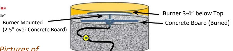
Pea Gravel fills the voids (for LP) and up and over the hardie board to the bottom of the burner. Then glass or lava rocks from bottom of the burner to 1/2 over the burner.
