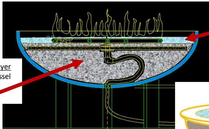
Natural Gas or Deeper Bowls - If using Nat Gas, or have a deeper bowl, can add extension and coupling to raise from 2" to 8". Mount FRMK to the bottom of the bowl/ pit to keep the burner straight up and down. Also, good if you are worried you'll heat up the hose.
