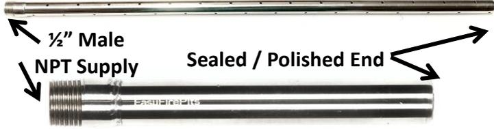
One Piece Design with 1/2" Male NPT Threads on one end and sealed and polished on other. 90 deg twin flame design (45° Left & Right of Top!)
