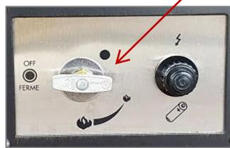
Mini-Needle Valve in place of Key Valve. Unscrew Nut and then unscrew T handle. Drill hole thru thin metal and install NV38 thru metal and reinsert T handle and screw back together
