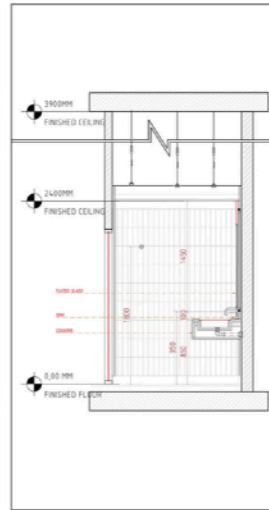
04 MALE FEMALE TOILET ELEVATIONS 03* SCALE: 1:20
