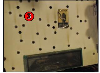
1 POWER OFF/UNPLUG machine 2 REMOVE backglass assembly 3 DISCONNECT all cables and REMOVE wood display panel. REMOVE all metal mounts from display panel for use on new panel.
