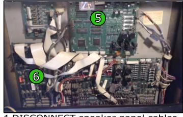
4 DISCONNECT speaker panel cables and REMOVE speaker panel
