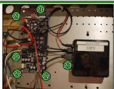
22 CONNECT speaker wires for speaker panel and cabinet subwoofer to audio controller board using included 4-pin connectors (if necessary)
