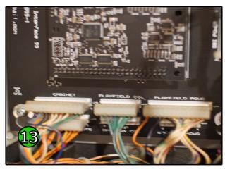
13 CONNECT all switch inputs to FAST controller
